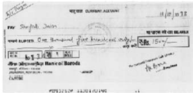
Figure 5.15: A Cheque Showing Magnetically-charged Characters that can be Read by an MICR Device
